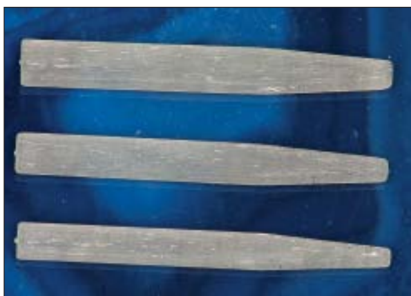
Fig 2a Representative image of oval glass fiber post specimens.
